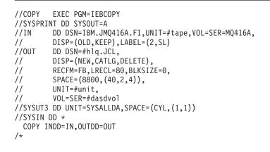
Figure 1. Load installation jobs
